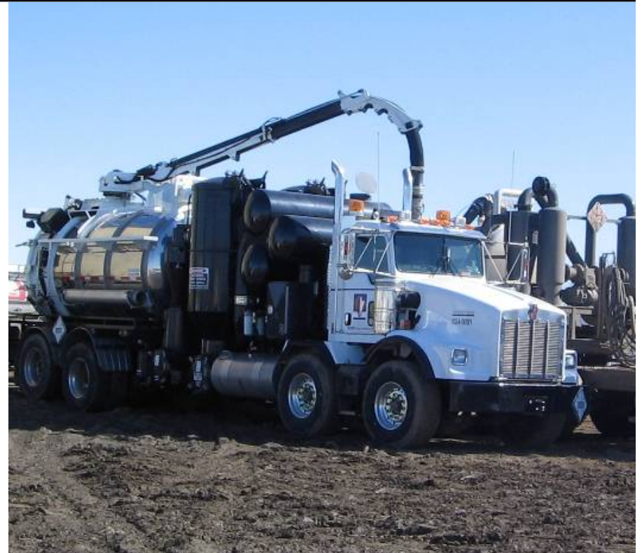
Pressure and vacuum unit – Oilfield Services
